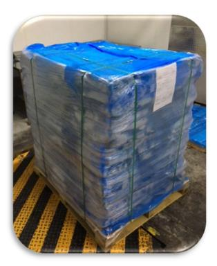
The product is delivered on wooden pallets of 120 X 100 Centimeters, with an average height of 110 cm. and an approximate weight of 500 kg is plasticized and strapped As shown in the image.
